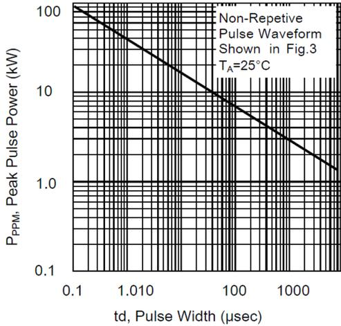
Figure 2. Pulse Derating Curve
