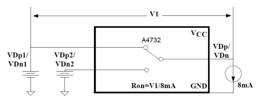
2. Test Circuit for Bandwidth,  $f_{3dB}$
