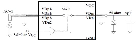
3. Test Circuit for Off Isolation, Viso
