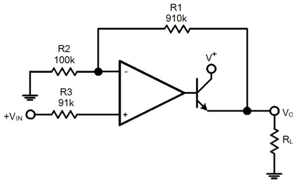
$V_0 = 0 V_{DC}$  for  $V_{IN} = 0 V_{DC}$ ,  $A_v = 10$
