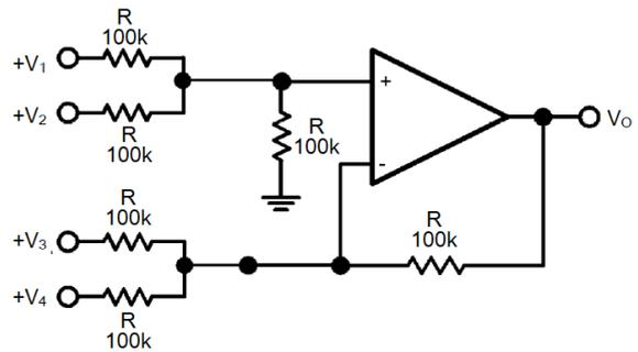
Where:  $V_0 = V_1 + V_2 - V_3 - V_4$ ,  $(V_1 + V_2) \geq (V_3 + V_4)$  to Keep  $V_0 > 0 V_{DC}$
