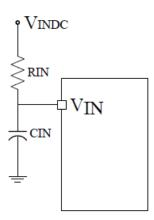
The R<sub>IN</sub>'s value must be between R<sub>max</sub> and R<sub>min</sub>.
