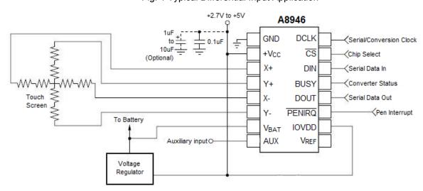
Fig. 1 Typical Differential Input Application
