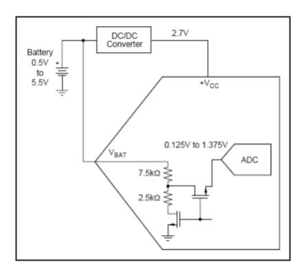
Fig. 5 Battery Measurement Functional Block Diagram
