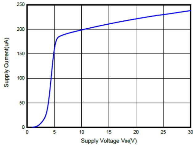
16. Shutdown Current vs. Supply Voltage
