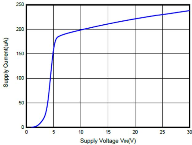
16. Shutdown Current vs. Supply Voltage
