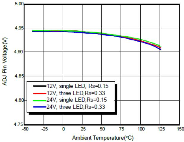
20. Voltage across  $R_{SENSE}$  vs. Temperature
