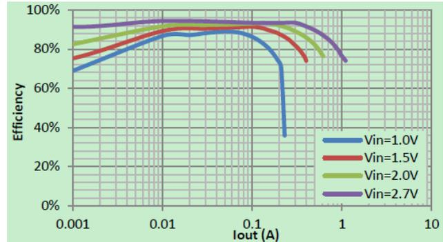
3. Efficiency vs. Output Current
