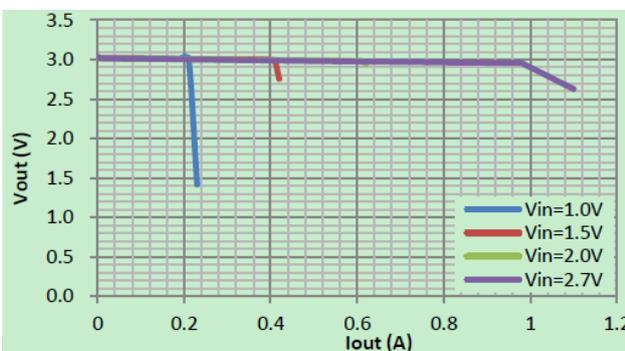
6. Output Voltage vs. Output Current
