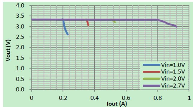
5. Output Voltage vs. Output Current
