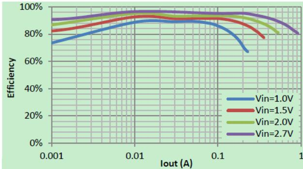
2. Efficiency vs. Output Current
