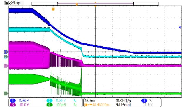
12. Trans response Waveform V<sub>IN</sub>=16V, V<sub>OUT</sub>=12V,
