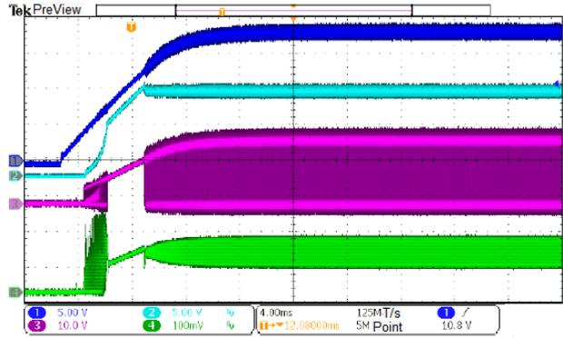
10. Shutdown Waveform with EN=V<sub>IN</sub>
