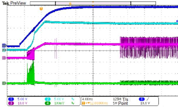
9. Start-up Waveform with EN=V<sub>IN</sub>
