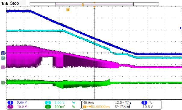
11. Shutdown Waveform with EN=V<sub>IN</sub>
