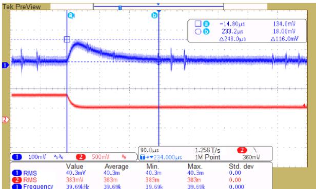
13. Trans response Waveform V<sub>IN</sub>=16V, V<sub>OUT</sub>=12V,
