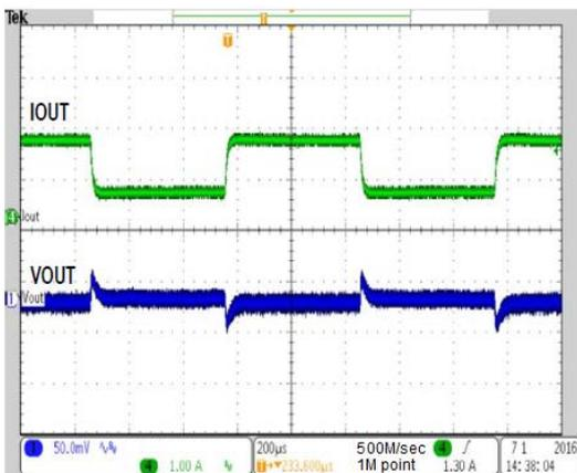
6.  $V_{IN}=5V, V_{OUT}=1.2V, I_{OUT}=0.5-2A$
