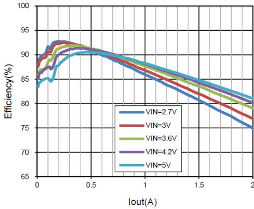
2. Efficiency vs.  $I_{OUT}$  @  $V_{OUT}=3.3V$
