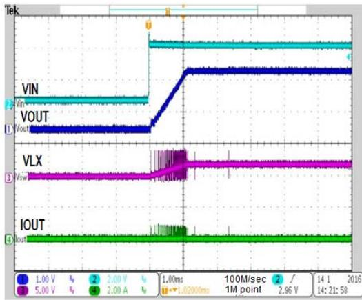
8.  $V_{IN}=3.6V, V_{OUT}=1.8V, I_{OUT}=2A$
