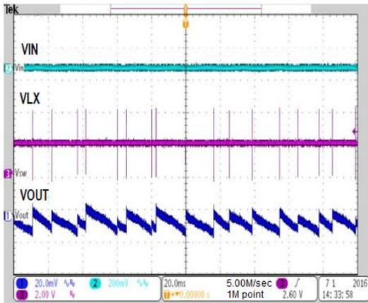
4.  $V_{IN}=3.6V, V_{OUT}=1.8V, I_{OUT}=2.0A$
