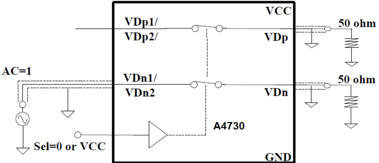
5. Test Circuit for Switch Times
