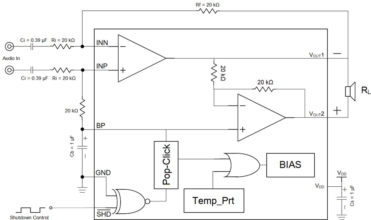
Figure. 2 A2203 Differential Amplifier Configuration
